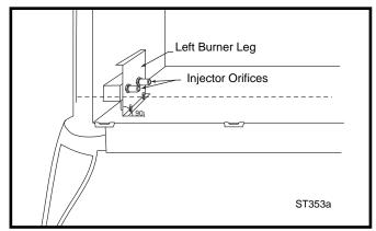
**Fig. 19** Be sure injector orifices remain at  $90^{\circ}$  to the base.
